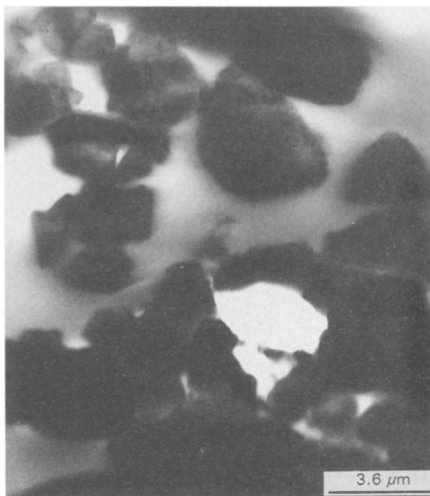
Figure 6 A transmission-electron micrograph for an 18 000 g mol -1 PDMS network filled with 30 wt % zeolite 4A.
